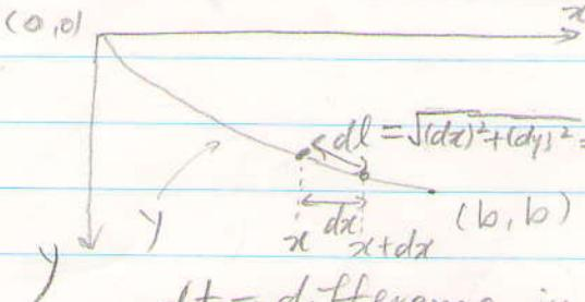
$$dl = \sqrt{(dx)^2 + (dy)^2} = \sqrt{1+y'^2} dx \quad \frac{1}{2} mv^2 = mgy \Rightarrow v = \sqrt{2gy}$$
