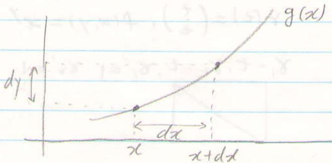
$$\begin{aligned} \text{length} &= \sqrt{(dx)^2 + (dy)^2} \\ &= \sqrt{1 + \left(\frac{dy}{dx}\right)^2} dx \\ &\sim \sqrt{1 + (y')^2} dx \end{aligned}$$
