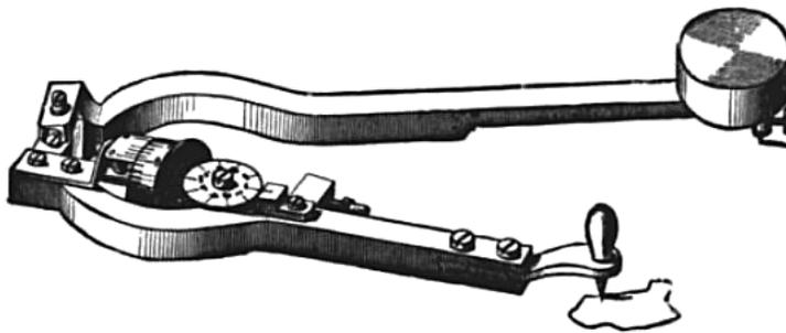
Wikipedia: Planimeter: A planimeter (1908) measuring the indicated area by tracing its perimeter.
